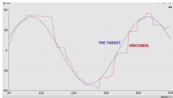
Figure 11. The sine wave target and performance of HMC5883L roughly oscillation
