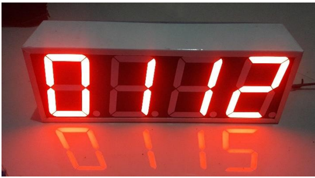
Fig. 4. 4-Digit Count-Up with 7-segment 5-Inch SM415001L
